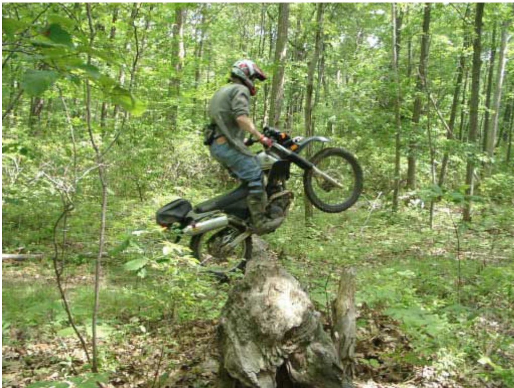
Trials style log crossing about 75% complete. Drive rear wheel into log while holding the front wheel up. Bash plate does not hit log during this maneuver.
