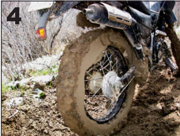
Severely caked mud like this can jam wheels and interfere with other mechanical systems. Clean up may be required to restore proper operation.
